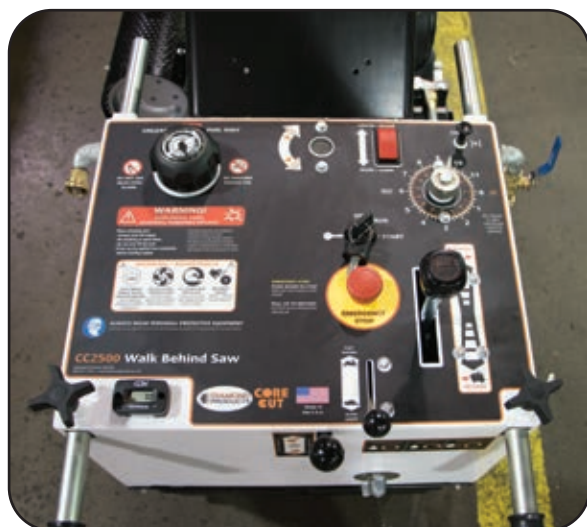
CC2500 control panel shown with optional raise/lower control switch
