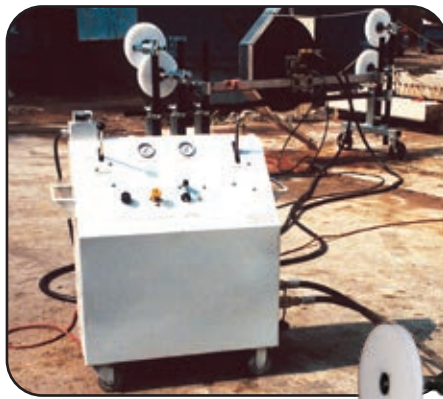
Wire Saw Control Station
