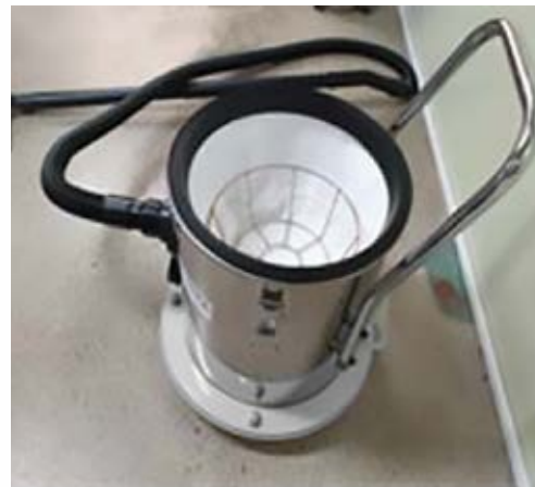
Pre-Filter for Dry Containment
