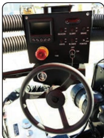
Digital Engine Panel, Fuel Gauge and E-Stop
